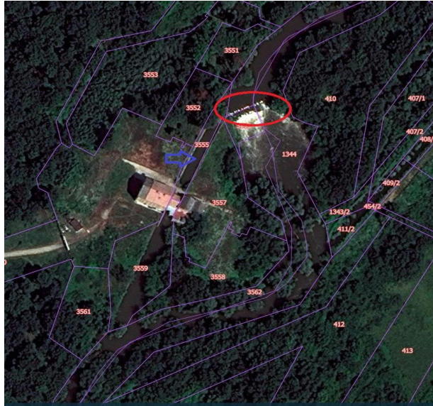
Figure 4: The mill by Straža. Red circle: the barrage, blue arrow: diversion channel
