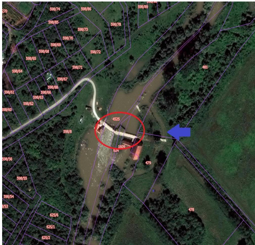
Figure 5: The mill by Vojvodinci village. Red circle: the barrage, blue arrow: diversion channel
